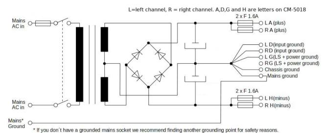
Diodes: >= 5A, >= 100V. Capacitors: >= 6600 uF, >= 50 VDC
